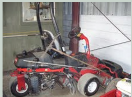
Toro 3250D Greens Mower - large, 3 cylinder, Briggs & Stratton 21 hp diesel engine provides exceptional performance required for greens and all surrounding areas.
